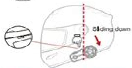
Install the host. Insert the raised buckle at the bottom of the host into the groove of the base.
