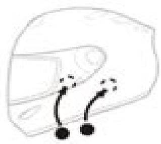
Open the inner lining on the ear position of the helmet attach the VELCRO loop.
